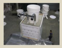
ASCE hosts an annual student Geo-Challenge competition. The competition requires students to design and build a mechanically stabilized earth wall model using paper reinforcement attached to poster-board facing. The design objective is to use the least amount of reinforcement needed to support the retained soil plus vertical and horizontal surcharge loads.
