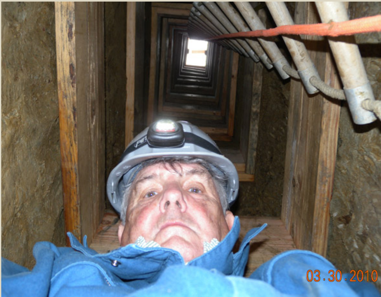
CalGeo Treasurer Rex Upp (Upp Geotechnology, Inc.) looks up from the bottom of a 41-foot deep hand-dug exploration pit as he studies a landslide in Saratoga.
